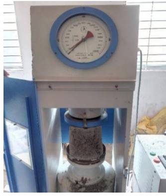
Figure 2. Compressive test on concrete
